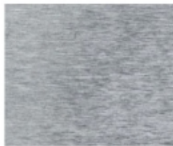
Surface finish: fine-machined, and grinded, Ra 0.4 \mu\text{m}
