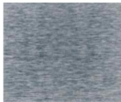
Surface finish: fine-machined, and grinded, Ra 0.2 \mu\text{m}
