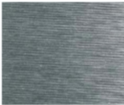
Surface finish: machined, Ra 1.2 \mu\text{m}
