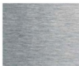
Surface finish: machined, Ra 0.8 μm
