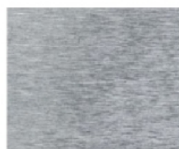
Surface finish: fine-machined, and grinded, Ra 0.4 μm
