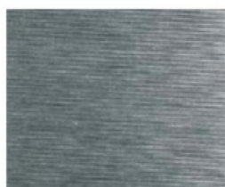
Surface finish: machined, Ra 1.2 μm
