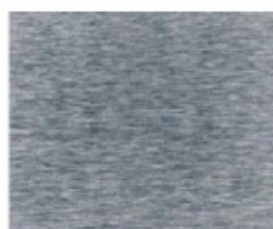
Surface finish: fine-machined, and grinded, Ra 0.2 μm
